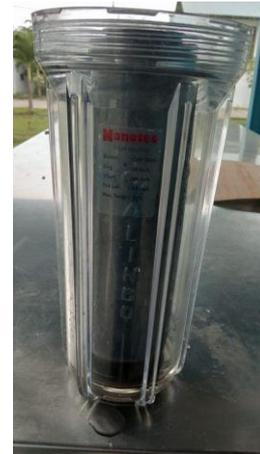
**Gambar 5.** Housing tempat cartridge filter
