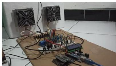
Gambar 7 Prototipe Sistem Monitoring Suhu
