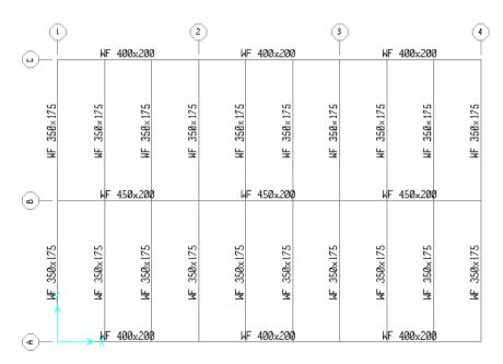
Gambar 1 Profile material denah lantai
