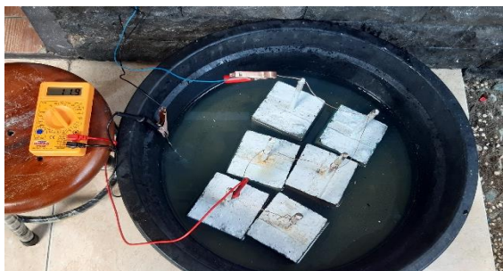
Gambar 6. Proses Pemberian Initial Corrosion
