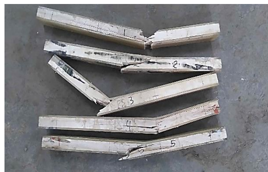
Gambar 10. Pola Kegagalan Balok Sandwich Panel HFRP Sengon
