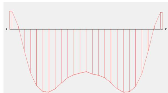
Gambar 6. *Model Penurunan Timbunan* (*Vertical disp.*=  $11.32 \times 10^{-3}$  m)
