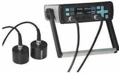
Gambar 3. Alat uji UPV, Proceq PUNDIT+
