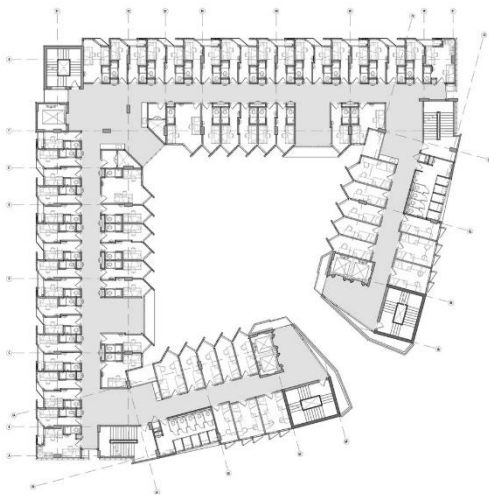
Gambar 12: Denah UBM Housing Sumber: https://www.archdaily.com
