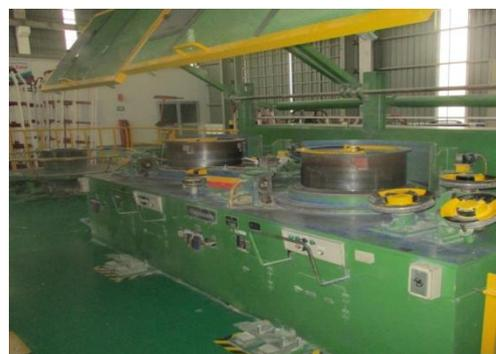
Gambar 3 Mesin *wire drawing*.
