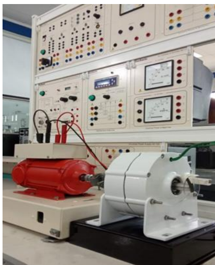
Gambar 2 Pengujian performa generator AC 3 phase di laboratorium
