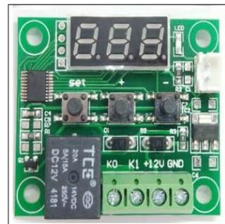
**Gambar 5.** Sensor Suhu Type w1209
