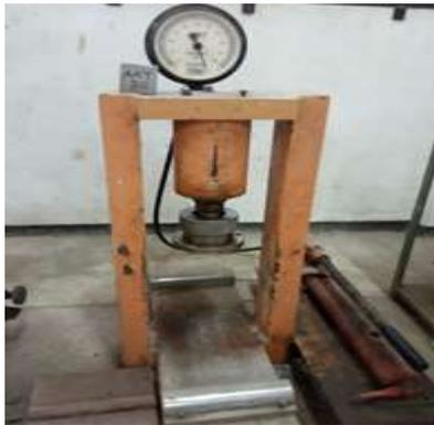
**Gambar 2.** CTM (*Compression Testing Machines*) Analogue
