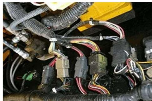
Gambar 1 Wiring Harness
