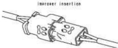
Gambar 2 *Defective Contact* antara *Male* dan *Female Connector*
