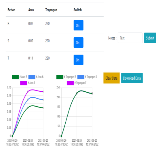
Gambar 8. Tampilan Web Percobaan beban lampu di phase R,S,T.
