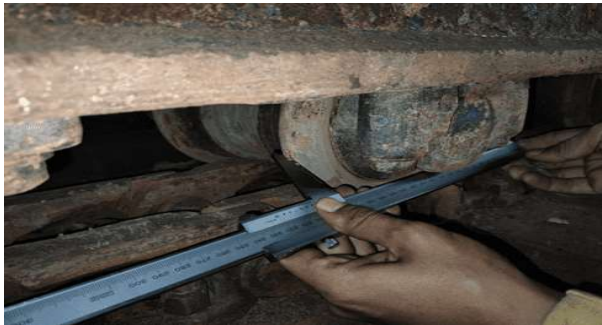
Gambar 14 Pengukuran diameter flange track roller
