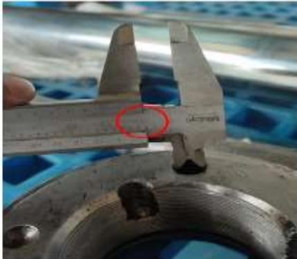
Gambar 10. Pengukuran Diameter Hole Piston Seal Cylinder
