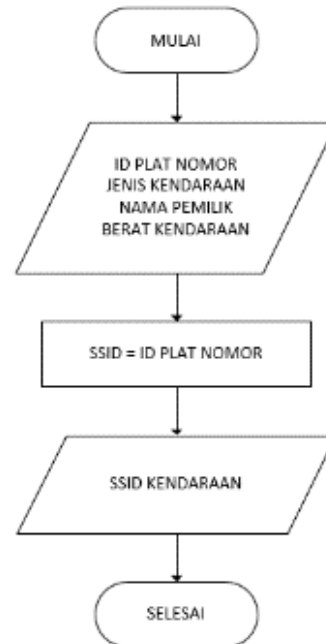
Gambar 10. Flowchart Client SSID
