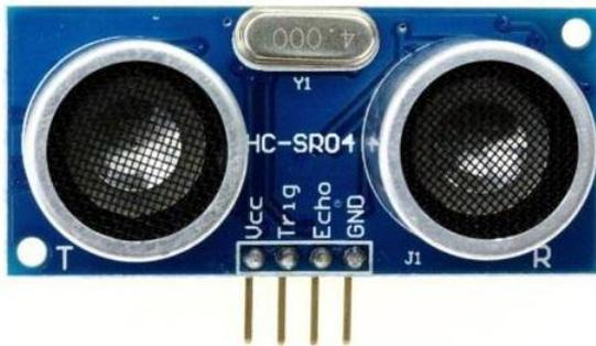
Gambar 1. Sensor ultrasonik HC-SR04
