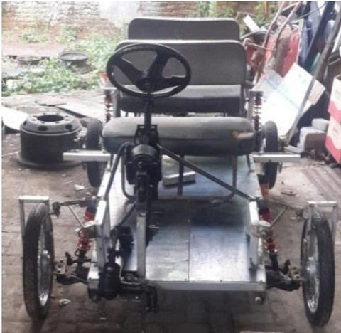
Gambar 1. Rangka Mobil Hybrid
