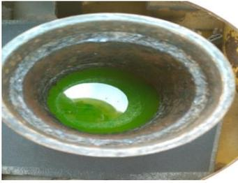
Gambar 2. Radiator Coolant Level
