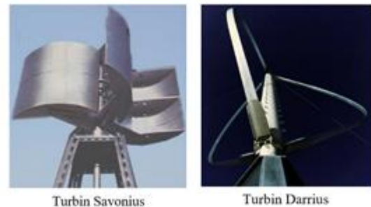
Gambar 1. Tipe turbin angin VAWT (Ambrosio & Marco, 2010)
