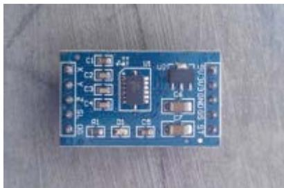
Gambar 7 Accelerometer type MEMS
