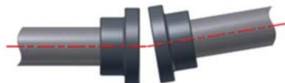
Gambar 3 Poros *missalignment* menyudut (*angular missalignment*).
