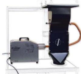
Gambar 1.2 TecQuipment AF17 open circuit wind tunnel dan ViCount Compact Smoke Generator (Gokcen Jurnal dkk, 2021).
