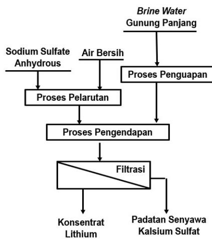
**Gambar 1.** Diagram Alir Percobaan
