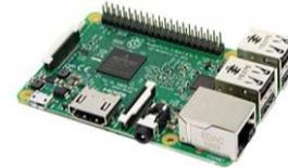
Gambar 4. Raspberry Pi 3 Model B
