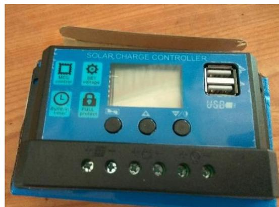
Gambar 10. solar panel charge control 12/24 volt
