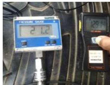
Gambar 3.67. Pressure and speed fan motor
