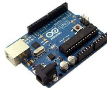
Gambar 2. Arduino Tipe UNO
