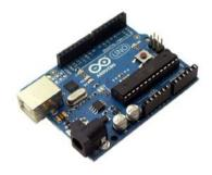
Gambar 2. Arduino Tipe UNO (Sensirion.com).
