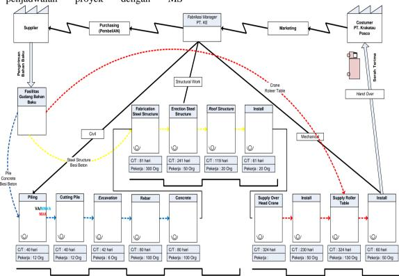
Gambar 2. Value Stream Mapping Structure WarehouseMC58 sampai MC62
