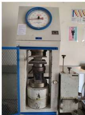
Gambar 4. Setting up Pengujian paving block
