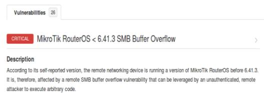
Gambar 12. *Vulnerability* Mikrotik RouterOS < 6.41.3 SMB Buffer Overflow.
