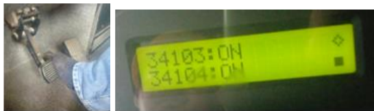
Gambar 8. Pedal service brake di tekan (normal)
