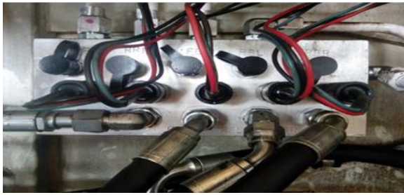
Gambar 11. Remove pressure switch
