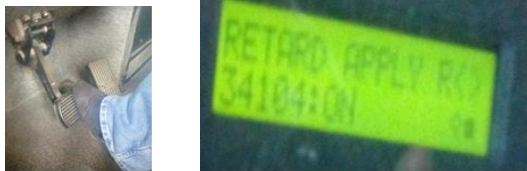
Gambar 12. Monitoring fungsi pressure switch
