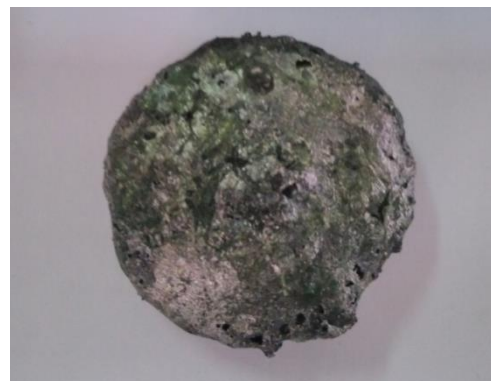
Gambar 1. Ingot CoCrMo 0,18 N hasil proses Arc Remelting Furnace
