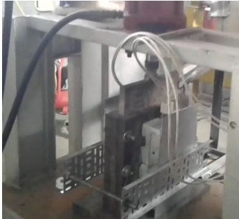
Gambar 9. Proses penekanan material coran.
