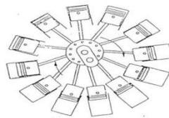
**Gambar 6. Motor Bakar Torak Radial. 10**
