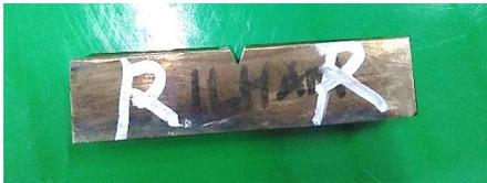
Gambar 3. Spesimen *disc brake* ASTM E23
