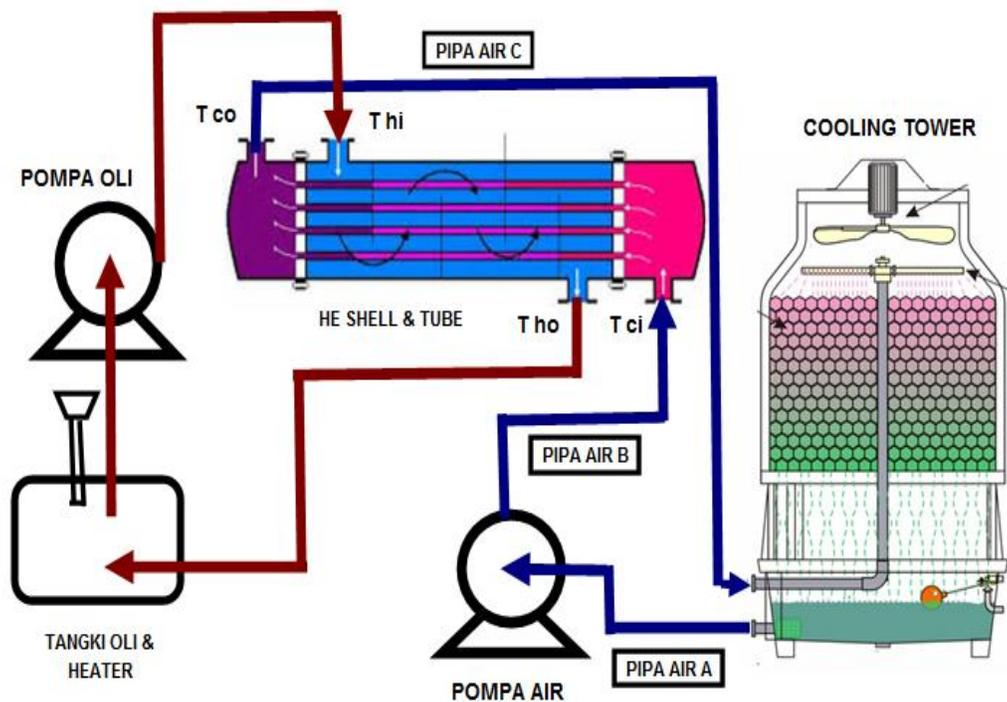
Gambar 4.1 skema instalasi pipa air heat exchanger
