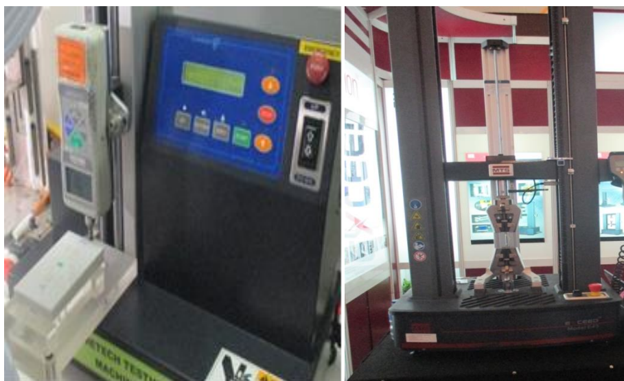
Gambar 2.7. Test Tarik Kunci Mesin Push Pull Tester Gambar 2.8. Universal Testing Mesin
