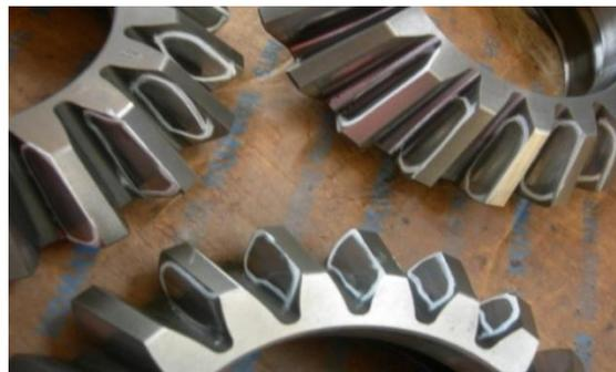
Gambar 11. *Differential Pinion Gear*
