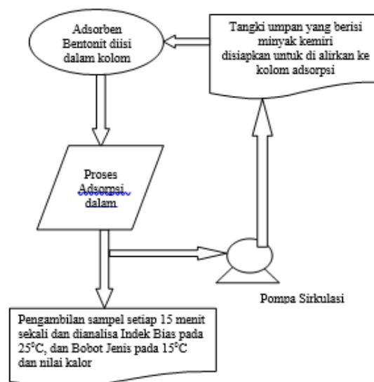
**Gambar 5.** Diagram Tahapan Proses Adsorpsi
