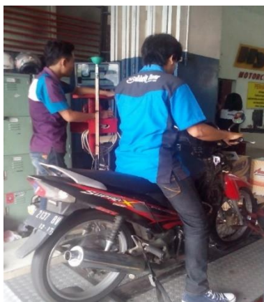
Figure 2. Performance test using dynamometer
