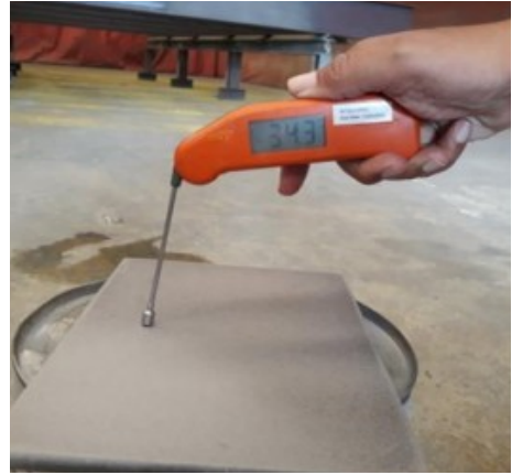
Figure 7. Check The Steel Temperature
