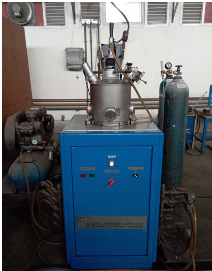
Figure 7. VAR machine with vacuum pump (left) and Ar gas cylinder (right).
