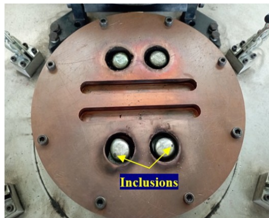
Figure 4. Metal oxide inclusions that float on top of the sample.
