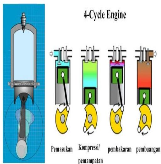
Gambar 1. Prinsip Kerja Motor Diesel
