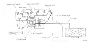
Gambar 6. Aliran Bahan Bakar Tipe In-Line
