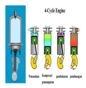
Gambar 1. Prinsip Kerja Motor Diesel
