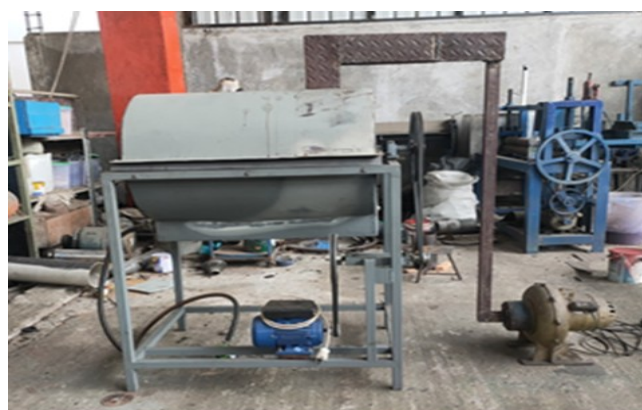
Figure 2. Horizontal Mill Type Coffee Dryer Using Suction Blower
