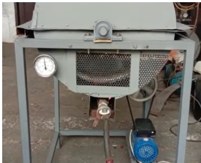
Figure 3. Front View of the Horizontal Mill Type Coffee Dryer, Including Temperature Gauge, Firebox, and Air Ventilation.
