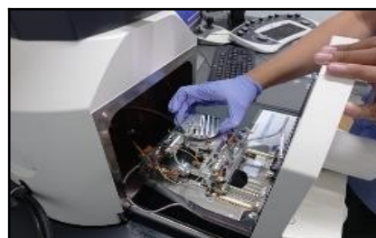
Figure 5. Placement of Specimens on the Testing Machine (SEM-EDX)
