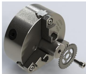
Figure 2. Illustration of CNC Lathe Chuck and Additional Attachments (Source: research documentation, 2024)
