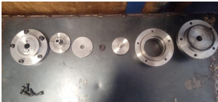
Figure 14. Collet Clamping Components After Machining (Source: research documentation, 2024)
