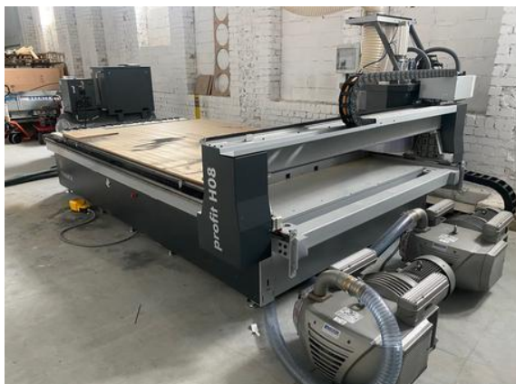
Figure 1. CNC Nesting Machine (Felder Format4 Profit H08) for specimen cutting (Source: Personal Documentation)
